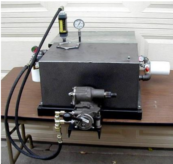
RPA 300 set up for testing gear boxes
