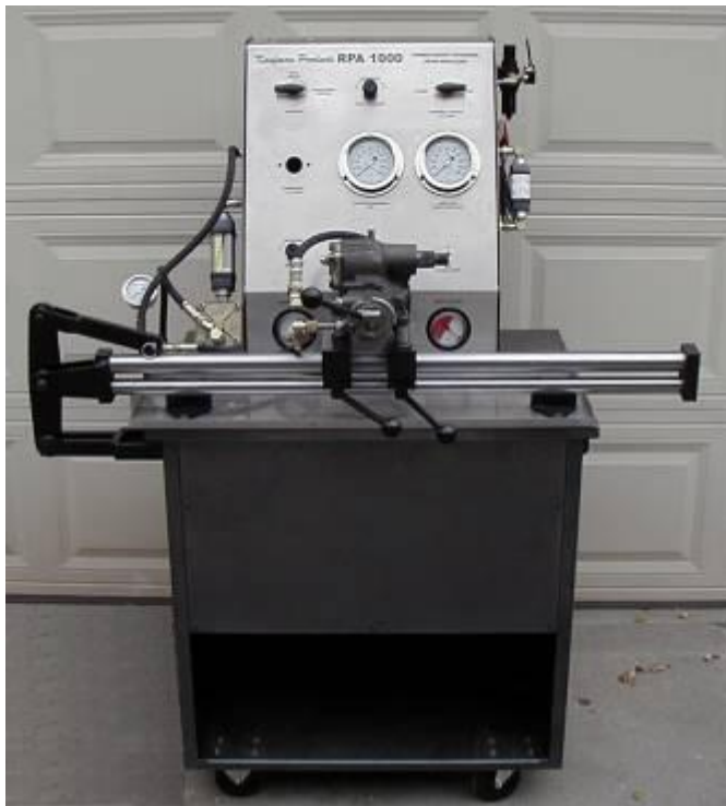
RPA 1000 set up for testing gearboxes
