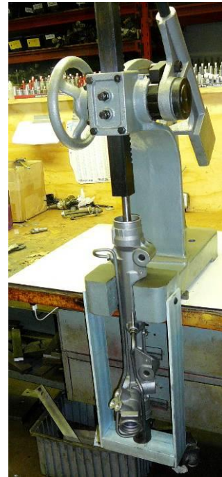
Pressing in Main Casting Seal in Assembly
