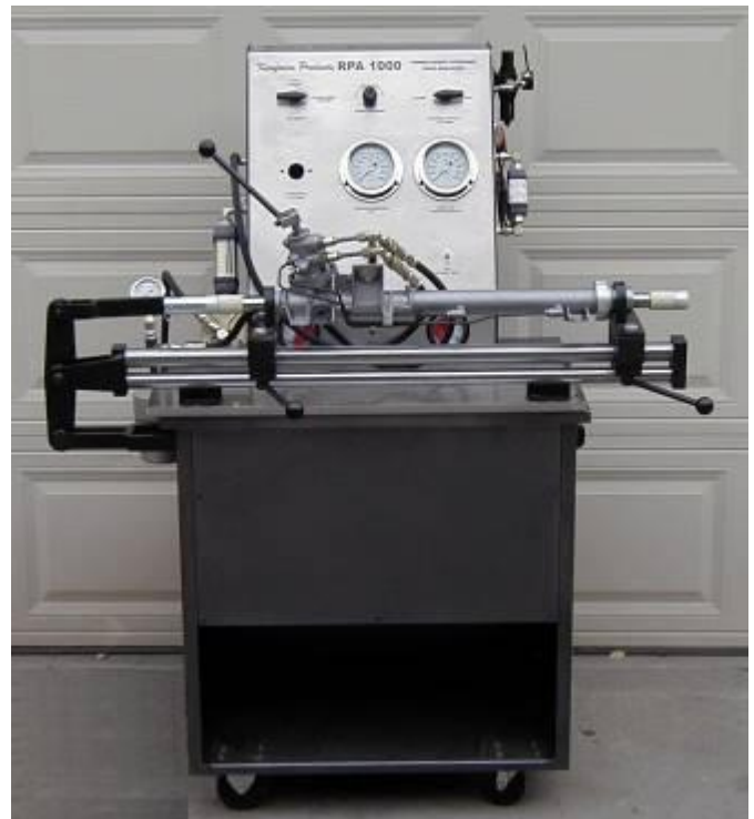
RPA 1000 set up for testing rack and pinion
